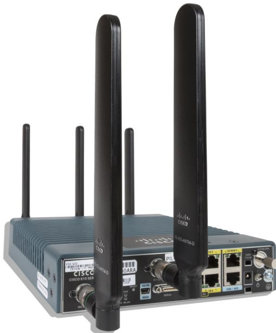
Figure 1. Cisco 819 Non-Hardened 4G LTE 2.0 Integrated Services Router with dual 802.11a/g/n radio WiFi
